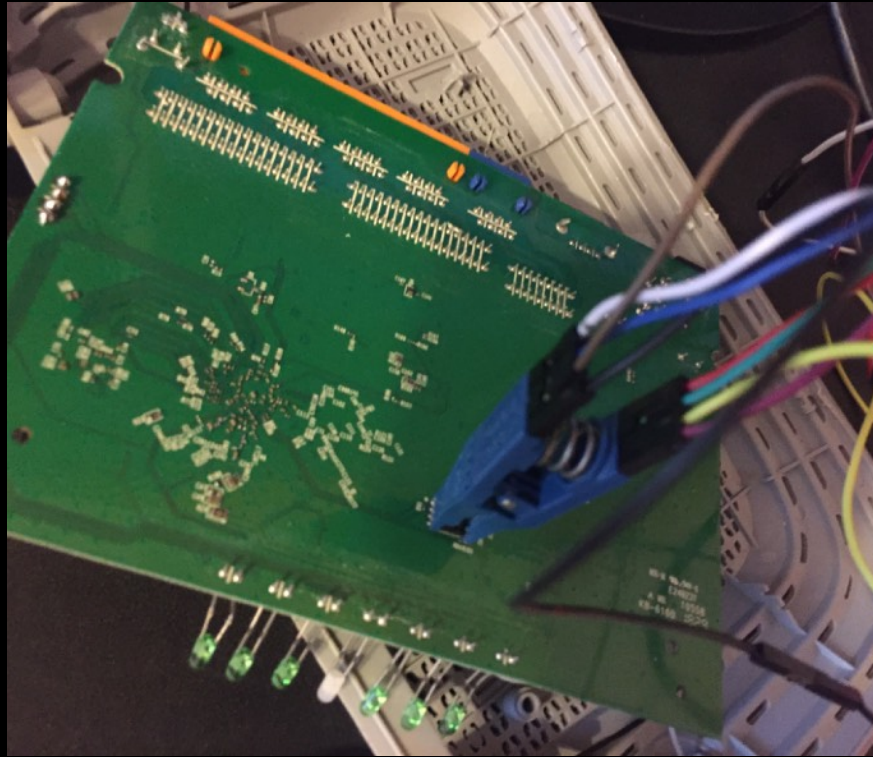
SOC8 clips connected to flash chip
