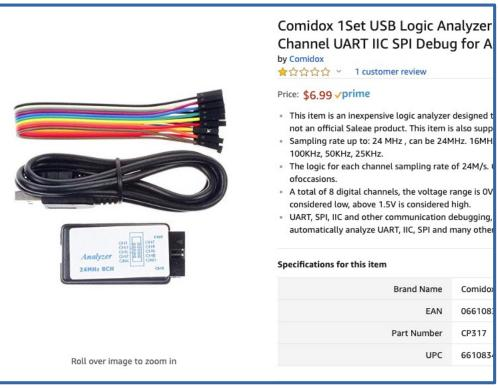
Super-cheap FX2 "LA" boards are really freaking cheap, and can capture up to 24MHz via Sigrok.
