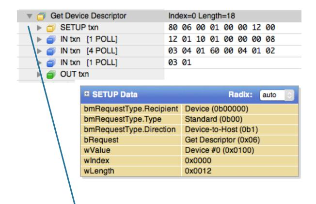
Each control transfer begins with a setup stage, describing the "command" (or "request") the host wants the device to perform.
