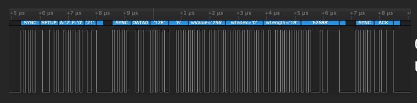
each control transfer is made up of three stages...
