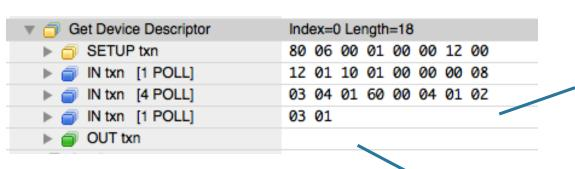
If the request has a non-zero length, the control transfer has a data stage during which data will be transferred in a single direction: either from host to device (OUT) or from device to host (IN).
