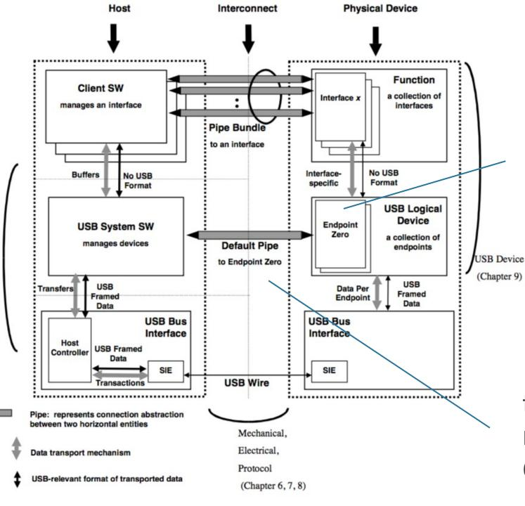
to support enumeration, every USB device must support a standard protocol on one of its channels
