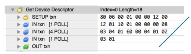
Each control transfer ends with a status stage, which confirms both sides agree that a transaction completed correctly.
