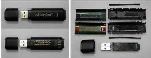
• Epoxy was removed using thermal method
