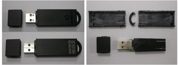
Epoxy was removed using chemical method
