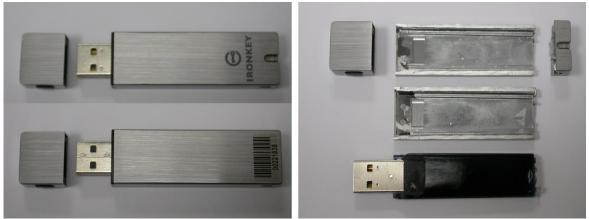
• Epoxy was removed using chemical method
