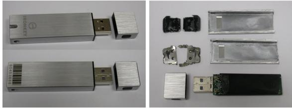
Epoxy was removed using thermal method
