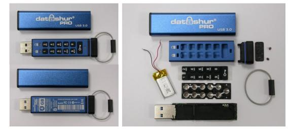
Epoxy was removed using chemical method
