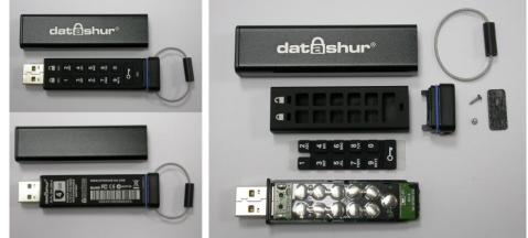
Epoxy was removed using chemical method
