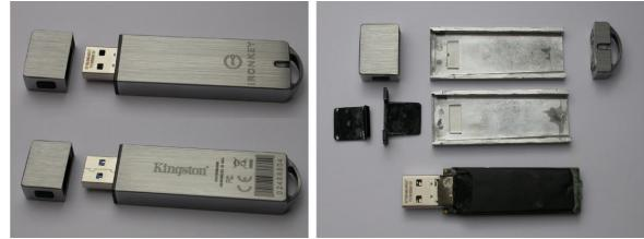
Epoxy was removed using thermal method
