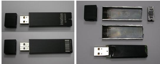
Epoxy was removed using thermal method
